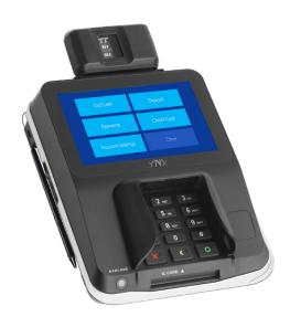
LYNX-9500 is the Multi ID-authentication terminal that supports every authentications service with ID verification from the contact card, live finger scanner, the contactless card, MSR and the electronic signature & PIN to the video file play as well as MOC, MOD and MOS.
