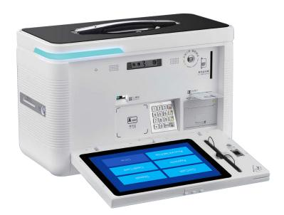
The Agent Unit device is a complete set of modules in the field of payment, which is assembled to provide teller services on site. This device can also serve as self-service according to different requirements of customers in absence of a teller.
